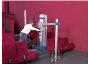
**4. The Movielift can still be moved with the rollers even after the basic unit has been built up. Thus it is child's play to move it to each desired position in the particular row of seats.**
