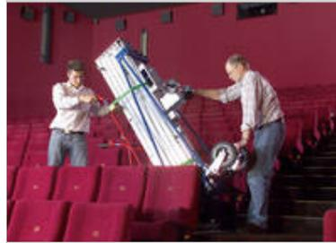
**2. The well thought-out Movielift can also be used in a simple manner between closely spaced rows of seats.**
