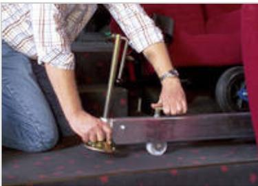
**5. After the desired position has been reached, the rollers are released and the Movielift is secured with the aid of its support feet.**
